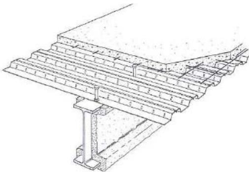
Figure 10: sketch of typical composite deck framing
