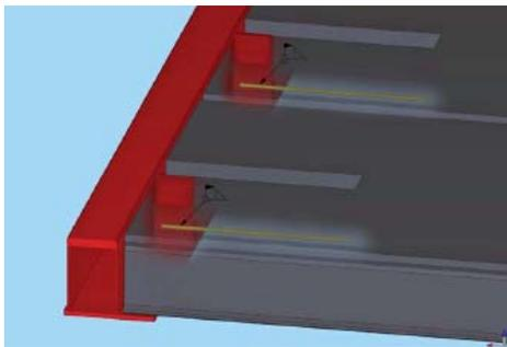
Figure 5: Principle connection of deck elements with one sided HSQ beam.
