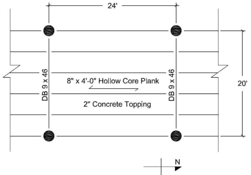
*Figure 15: Framing Layout, Bay A*
