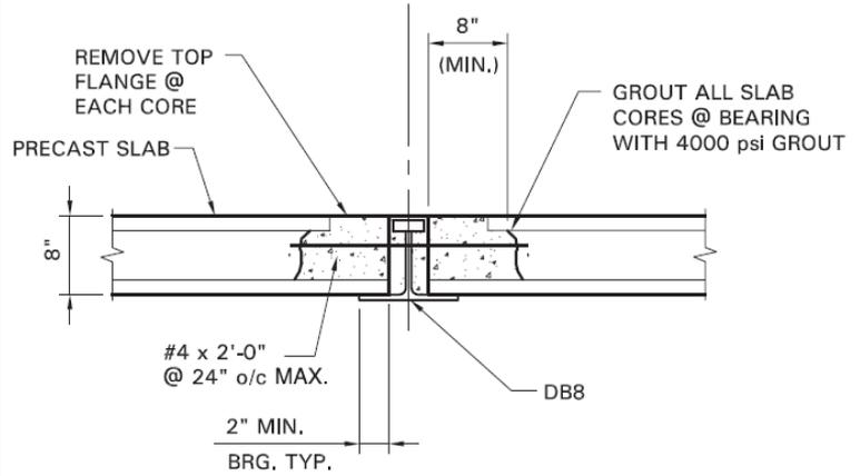
**TYPICAL SECTION: 8" GIRDER-SLAB® SYSTEM**
