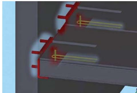
Figure 6: Principle connection of deck elements with interior concrete wall.
